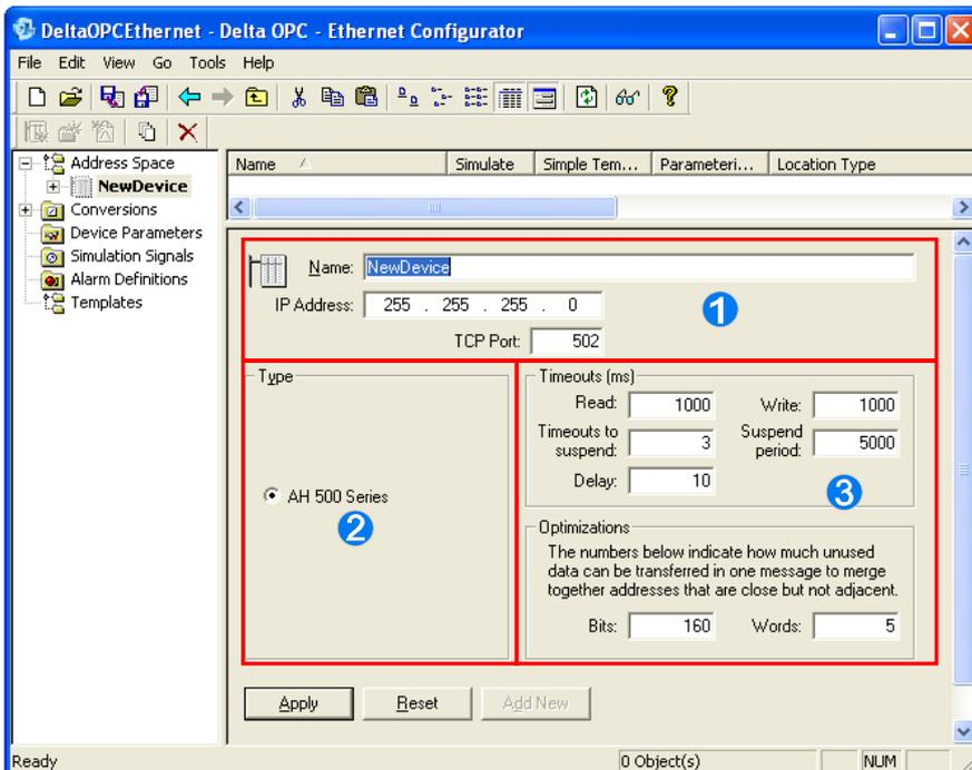
Figure 3-9 Setting a device (Delta OPC - Ethernet Configurator)
