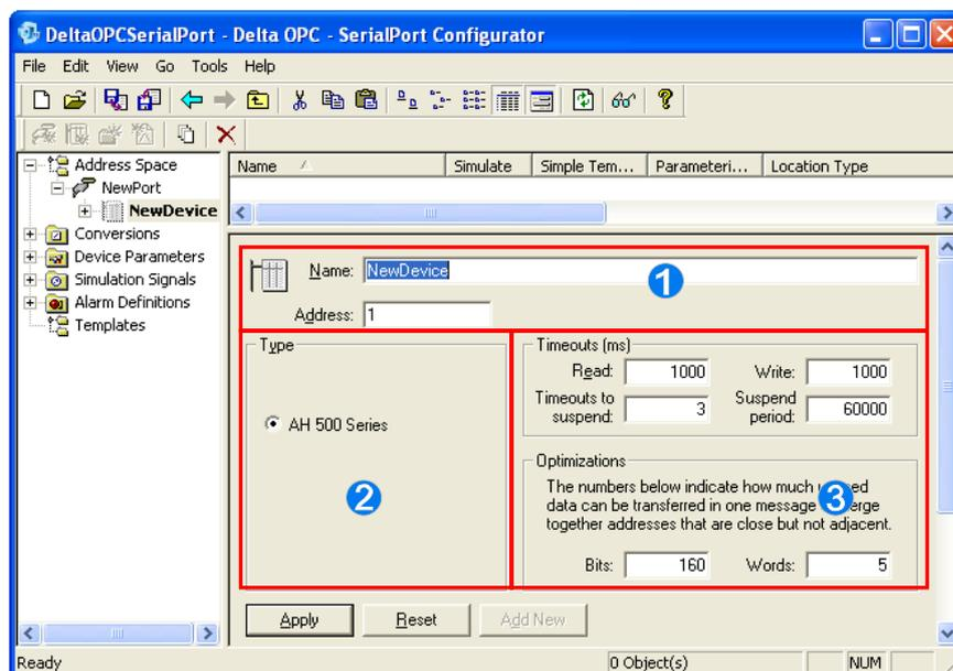
Figure 3-7 Setting a device (Delta OPC - SerialPort Configurator)
